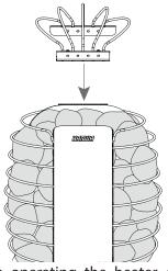
Before operating the heater, fill the heater with rocks and install the rock guard.
