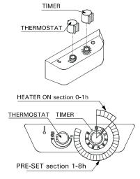
**TIMER:** To activate the heater, use the timer switch, and the indicator lights will illuminate. The timer features two scales: the "instantly on" section (0–1 hours) to star heating and the "pre-set section" to delayed start up to 8 hours.
