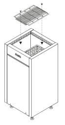
Before operating the heater, fill the heater with rocks and install the safety grid.
