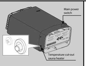
The heater's temperature protection devices:
