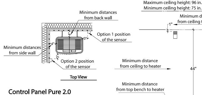
•The control panel position can be installed inside or outside the sauna room, the minimum distance when is installed inside the sauna is 12" between heater and control panel and the max height is 36" distance off floor.
